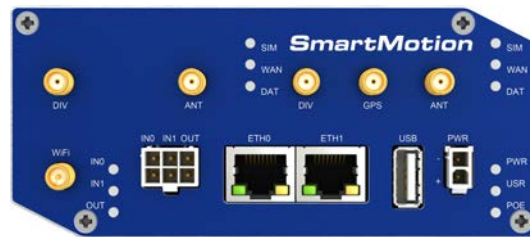
Figure 7: Version with WiFi module
