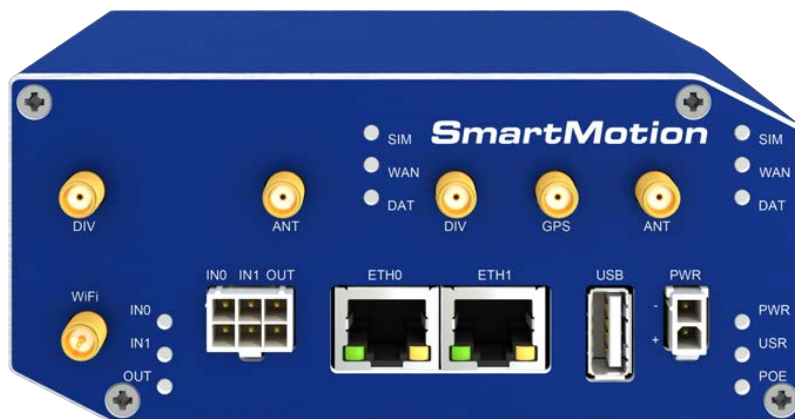
Figure 12: SmartMotion front panel
